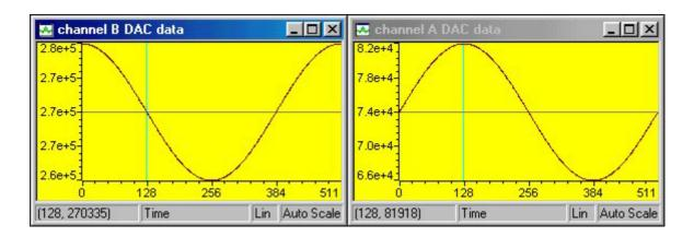
The graphs show the data that will be output to the DACs. Notice the vertical bar marking the 128<sup>th</sup> sample. For the purposes of this demonstration you can connect the DAC outputs to the ADC inputs for each channel. This is OK for the HERON-IO2 as the output and input voltage ranges match.
