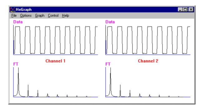
When you have changed the outputs to be square waves, and enabled the Frequency plot you should see the graph above.
