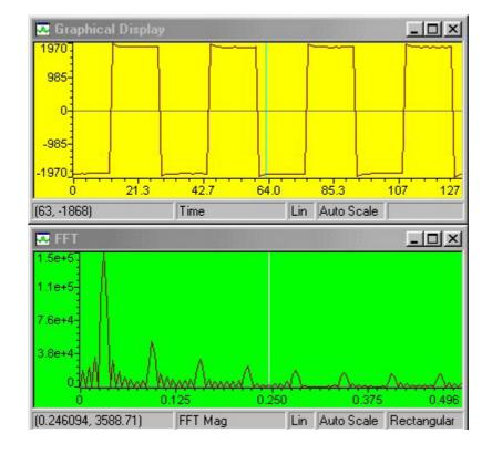
Again the square wave is not perfect as the system bandwidth is not infinite, but now you can see the various frequency harmonics that are contained in the square wave signal.
