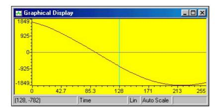
The array "shortdata" actually contains both channels of ADC data, with A in the first 128 samples and B in the second 128 samples. In the graph above you cannot see the change, which is because 128 samples of the Sin exactly lines up with the first 128 samples of the Cosine. Look at the original graphs to check it.
