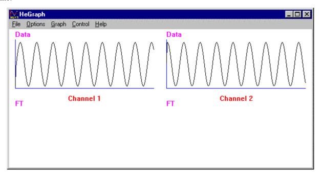
After selecting File -> Start, the 'hergaph' program should display a waveform as shown above. If you don't see this, verify that you have connected your inputs to your outputs correctly. Also, as already stated you must have successfully loaded the correct HERON-IO2 bit-stream for example 2. Verify that the "Done" LED on the HERON-IO2 is switched off and the User LED4 is flashing slowly.
