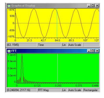
The frequency spectrum is "nearly" a single point, the smaller items are being introduced by the sampling process on the output of the DACs and the input of the ADC.
