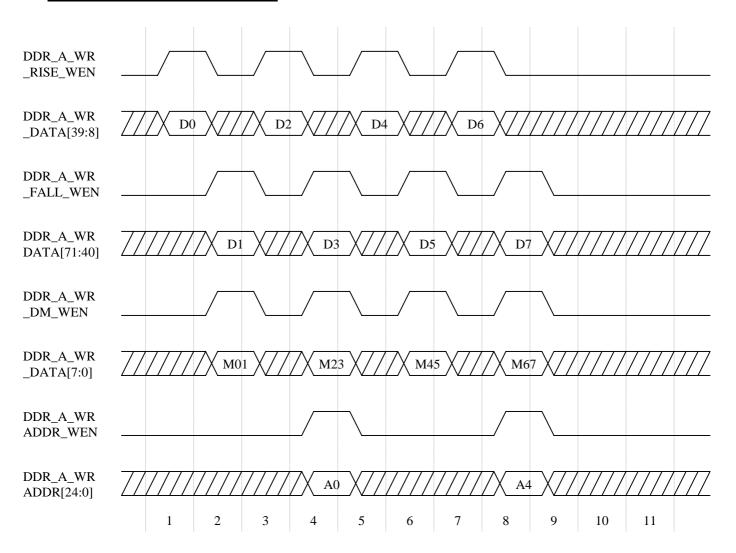
In the above diagram eight words are written to memory at A0 to A7. There are four FIFOs involved in this operation. The rising data FIFO, the falling data FIFO, the data mask FIFO and the address FIFO. It is assumed that all FIFO flags are checked such that no time are any of the FIFOs full. This is done using the FIFO flags presented by the DDR memory interface component.
