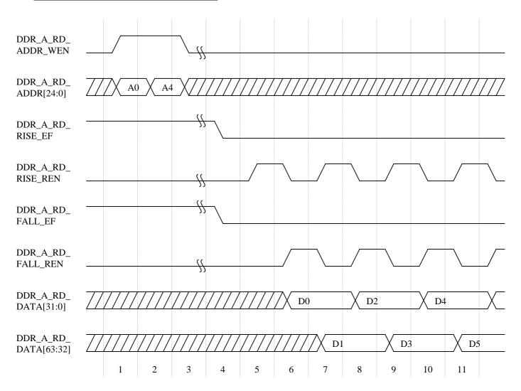
In the above diagram eight words are read from memory at A0 to A7. There are three FIFOs involved in this operation, the rising data FIFO, the falling data FIFO and the address FIFO. It is assumed that the address FIFO flags are checked such that no time is the address FIFO full. This is done using the FIFO flags presented by the DDR memory interface component.
