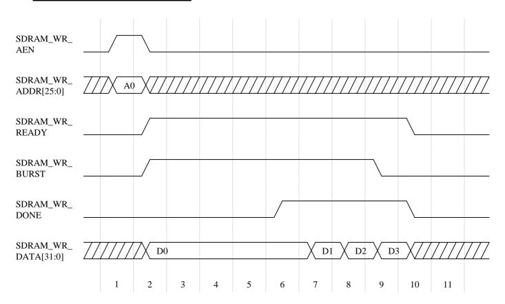
In the above diagram four words are written to memory at A0, A0+1, A0+2 and A0+3. The first operation performed is to set the write address by asserting the  $SDRAM_WR_AEN$  along with a valid address on  $SDRAM_WR_ADDR$ . This must be done before the  $SDRAM_WR_READY$  signal indicates data is ready to be written at that address.
