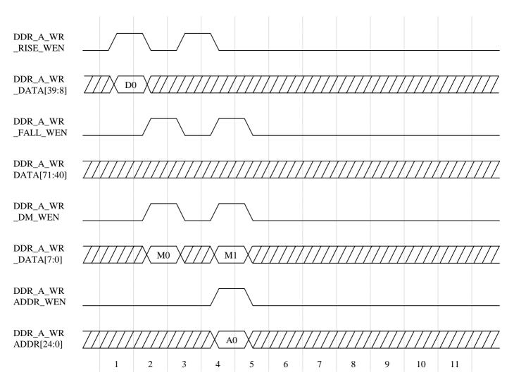
The data mask function is necessary when trying to write to less than four locations of memory. For normal operation, data would always be written in groups of four words as this allows the DDR memory interface to burst at the most efficient rate. This section describes a situation where only word is to be written to memory.
