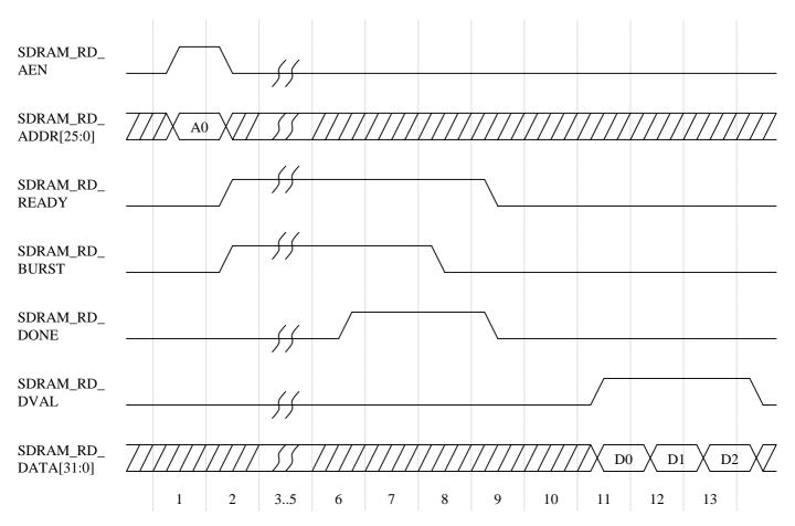
In the above diagram three words are read from memory at A0, A0+1 and A0+2. The first operation performed is to set the read address by asserting the  $SDRAM_RD_AEN$  along with a valid address on  $SDRAM_RD_ADDR$ . This must be done before the  $SDRAM_RD_READY$  signal indicates data is ready to be read at that address.
