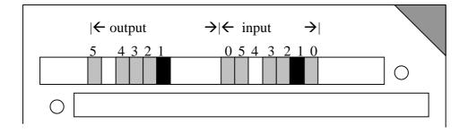
These jumpers are used to select the default routing of FIFO 0 on the Carrier card.
