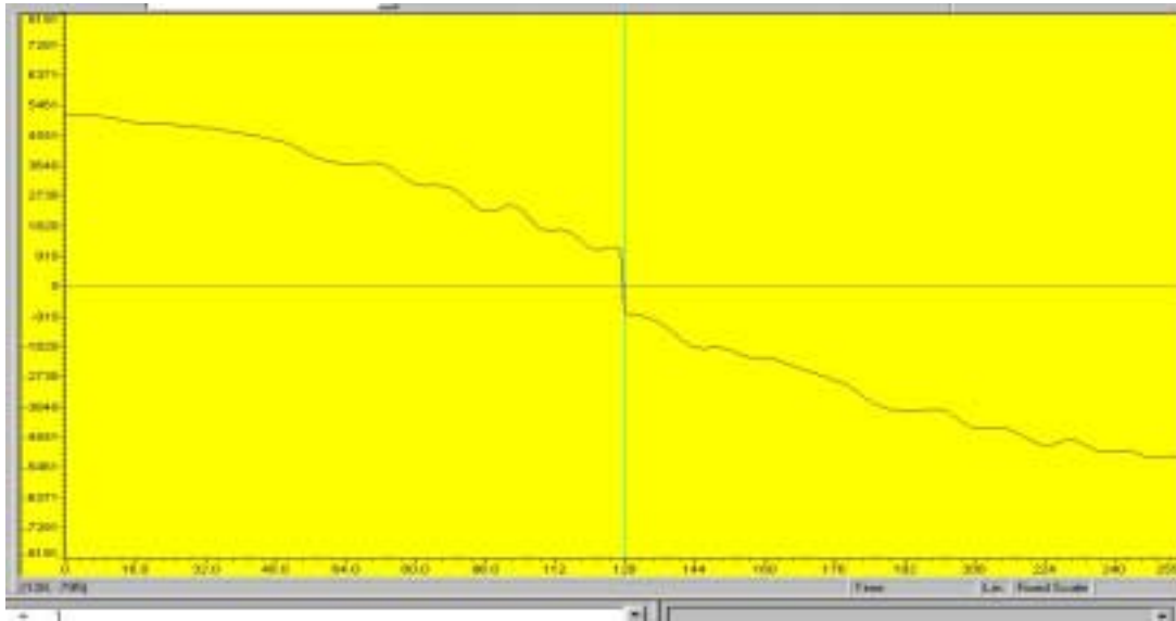
FIGURE 10 – DDC Output with Poor Jitter
