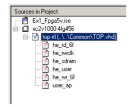
In the case of the FPGA5v1 example conversion, after adding 'top.vhd' we can now see 6 more design entities are needed. One of these entities is the User-Application level of the design which contains the VHDL that makes this example the getting started example, Example1. The other entities shown are part of the Hardware Interface Layer and are found in the 'Common' directory.
