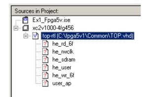
In this picture we can see that the path shown for 'top.vhd' is absolute. That is, it shows the complete path. The project needs to be changed to use relative path information. To do this, left click on the entity 'top'. With top selected, right click to bring up a menu and select 'Toggle Paths'.
