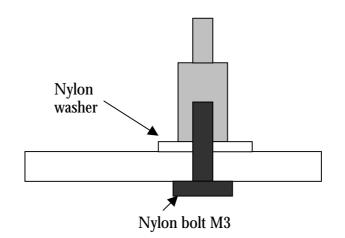
This means that when the HERON modules are fitted, the male part of the pillars helps to properly align the module as it is pushed into the sockets. Then an M3 nylon nut can be fitted to the top of the module to firmly retain it in each of four places.
