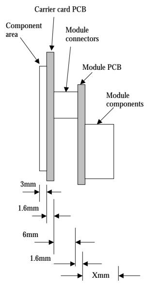
In PCI, ISA, VME and cPCI systems the normal slot spacing is a little more than 20mm, making a sensible single slot card be 20mm. So, in order to allow a single slot assembly a HERON module would require X to be less than 7.8mm.
