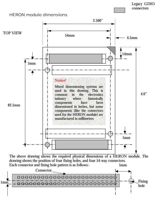
The fixing holes have a diameter of 0.125" providing a clearance hole for an M3 fixing, and the connectors use a hole diameter of 0.030", which is large enough to accept the pins.
