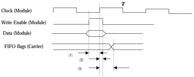
There will be faster versions of the FIFO interface over time, but the initial interface will have a maximum clock frequency of 67Mhz. As faster interfaces are implemented this document will be updated with the timings used by them, it is however expected that a slower module will always be able to work with the timings of a faster Carrier card.
