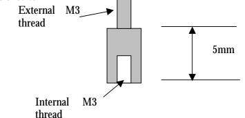
These are fitted to the carrier board using an M3 nylon bolt from the non module side of the carrier, and there is a nylon washer fitted between the metal pillar and the module side surface of the PCB. i.e.
