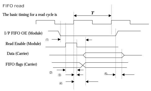
There will be faster versions of the FIFO interface over time, but the initial interface will have a maximum clock frequency of 67Mhz. As faster interfaces are implemented this document will be updated with the timings used by them, it is however expected that a slower module will always be able to work with the timings of a faster Carrier card.
