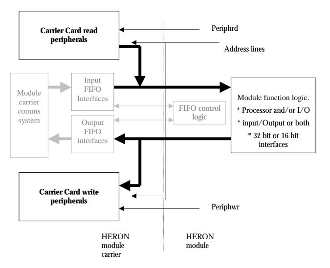
The diagram demonstrates the sharing of the HERON module data busses with the FIFO interfaces. This means that the peripheral accesses cannot take place at the same time as the FIFO accesses. Please note that to perform a peripheral read cycle the FIFO output enables must be inactive to prevent the FIFOs from driving the module's input data bus.
