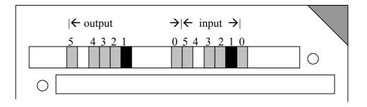
These jumpers are used to select the default routing of FIFO 0 on the Carrier card. This is to enable the actual source of the boot stream to be set up, even before the application starts and configures the system connectivity to be used.
