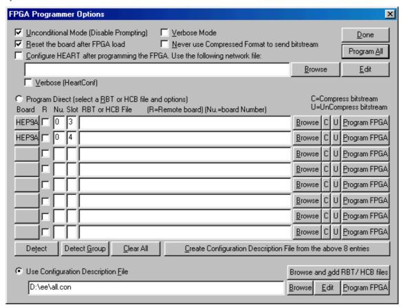
Then you can type in the path and bit-stream file name, or use the browse button to navigate to the correct file: -
