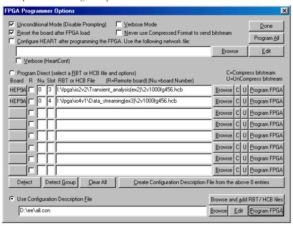
Then you can use the program FPGA button next to that line to configure all devices that appear in that file.
