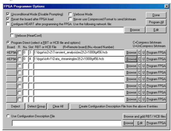
Now the Program FPGA button can be used to program a single FPGA, or the Program All button used to program all FPGAs in your list. The 'Board', 'Nu' and 'Slot' fields indicate what board and slot the detected module is on. You can manually change the fields.
